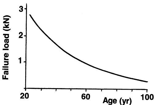
Figure 48.3. Variation of failure strength of bone–anterior cruciate ligament–bone preparations with age. From Woo et al. [5] with permission.
