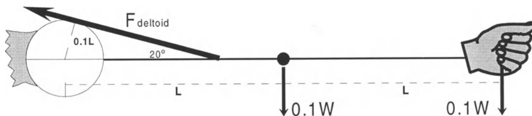
Figure 38.7. Loading example of the horizontal arm. The hand is carrying a weight of 10% body weight ( 0.1W ) and the weight of the arm itself ( 0.1W ) acts through the center of the limb. The two loads provide a clockwise turning moment that must be balanced by the anticlockwise moment of the deltoid force for the arm to remain abducted in equilibrium.
